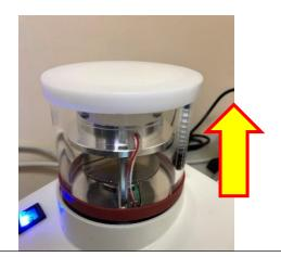
向上輕拿玻璃蓋、勿撞中間金屬! CAREFULLY move the glass chamber upward. Don't hit the metal part.
